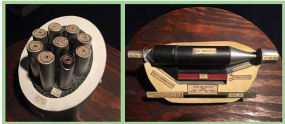
Historic models from James Powell’s invention of Particle Bed Reactor.
