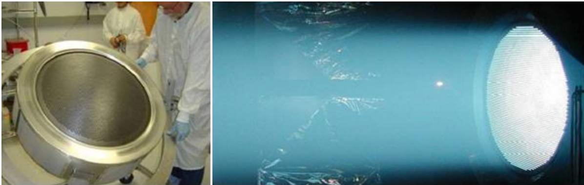
Figure 3. The 20-kW Nuclear Electric Xenon Ion thruster System (NEXIS) developed at NASA-JPL for the Jupiter Icy Moons Orbiter (JIMO), later cancelled (courtesy of NASA)
