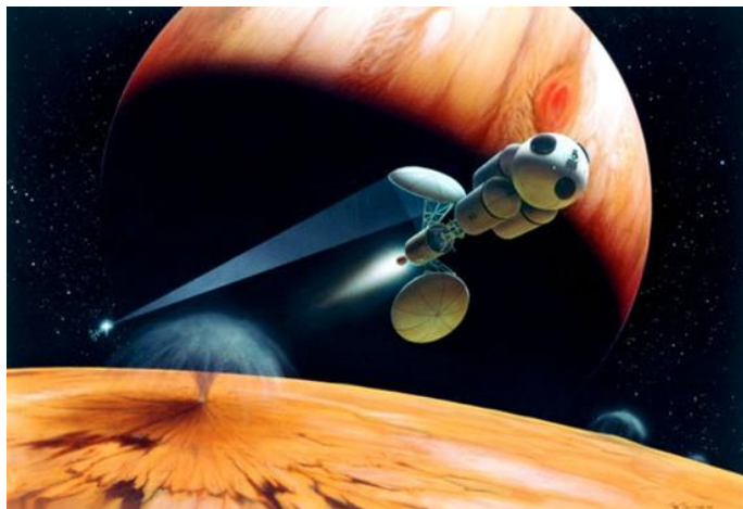
Figure 7. Left: a laser beam illuminates the PV collector of a high-power EP spacecraft (source: http://www.projectrho.com/public_html/rocket . Right: array of 21 laser emitters generate and steer a combined beam (Courtesy of DARPA)
