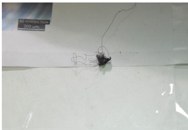
Figure 3. 50 µm diameter ^6\text{Li} wires made at the Y-12 National Security Complex..
